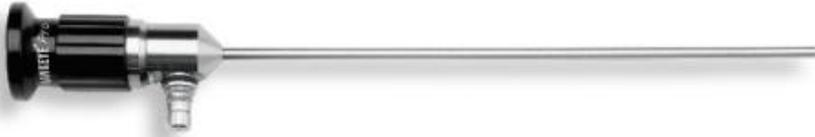
Choose a rigid Borescope when the entry path is straight. Rigids offer the higher resolution, better image quality, more durability and are less expensive than flexible fiberscopes. Hawkeye Classic and Pro Rigid Borescopes have DOV's of 0°, 30° and 90°. Hawkeye Blue Rigid Borescopes offer a wider selection of DOV's and lengths.
